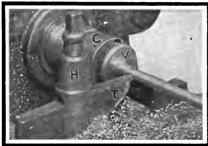
Fig. 8—Method of rough turning the valve after having both ends centered
